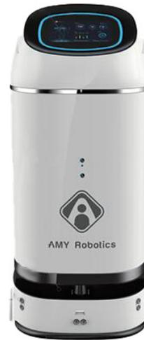
Autonomous, automatic disinfection robot with dry-fog mist nozzle system spraying disinfectant hydrogen peroxide solution
